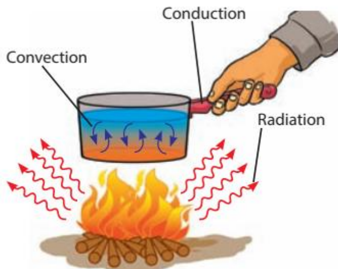
Figure 14.29 ▲ Methods of heat transfer
